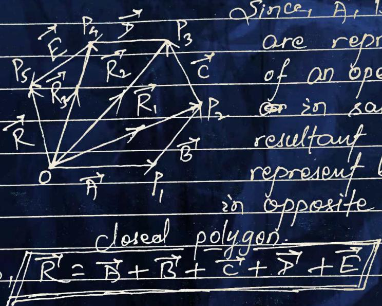
Since,  $\vec{A}, \vec{B}, \vec{C}, \vec{D}$  and  $\vec{E}$  are represented by sides of an open polygon  $OP_1P_2P_3P_4$  in same order and its resultant vector  $\vec{R}$  is represented by the side  $OP_5$  in opposite order of this closed polygon.
